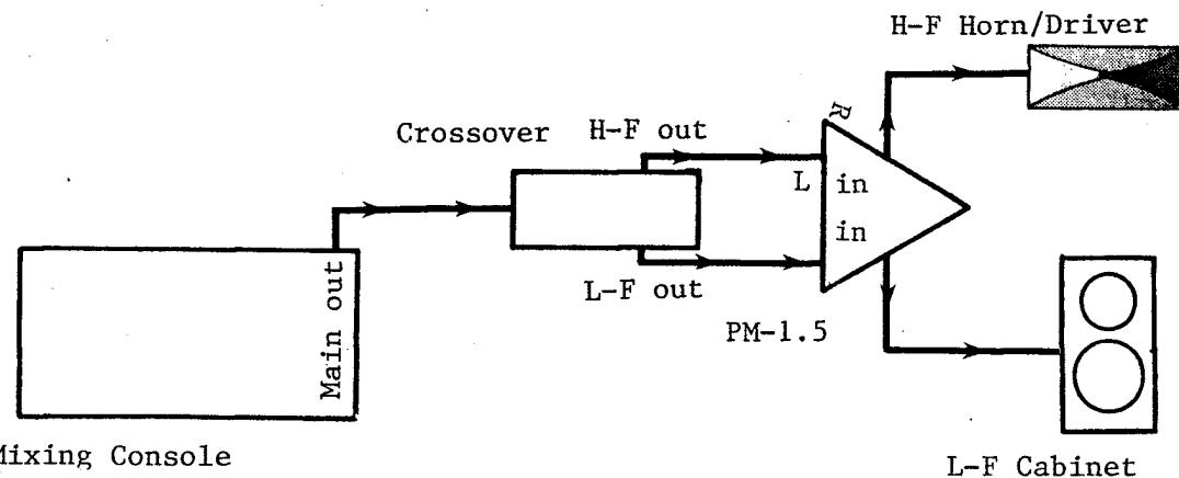
The diagram shows the connections for such a system. Here, the high-frequency output of the crossover is connected to the left-channel input of the PM-1.5, and the low-frequency output of the crossover is connected to the right-channel input. Connections are made between the respective loudspeaker elements and the amplifier's output terminals. Of course, the loudspeakers in this set-up, like any dual-channel set-up, must have a nominal impedance of  $4\Omega$  or greater.
