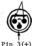
Note: Failure to connect Pins 1 and 2 will result in an approximate 50% reduction in gain. This is done automatically when using the TRS jacks to supply unbalanced drive signal to the PM-1.5 with standard  $\frac{1}{4}$ -inch phone plugs.
